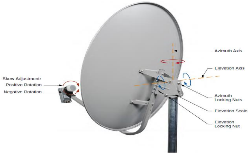
Antenna look-angle adjustments.
